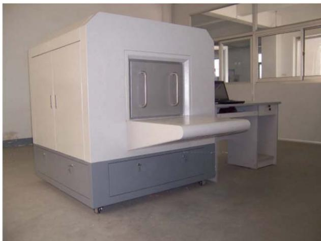
The baggage scanner developed at CRIRP.
