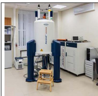
Bruker 400 MHz WB Avance NMR spectrometer is dedicated to the studies of samples in solid state: crystallines, powders, weakly ordered materials, gels, liquid crystals, amorphous compounds, nanostructures (zeolites, silicates) etc. The spectrometer allows one to study diffusion processes and obtain micro-tomographic image
