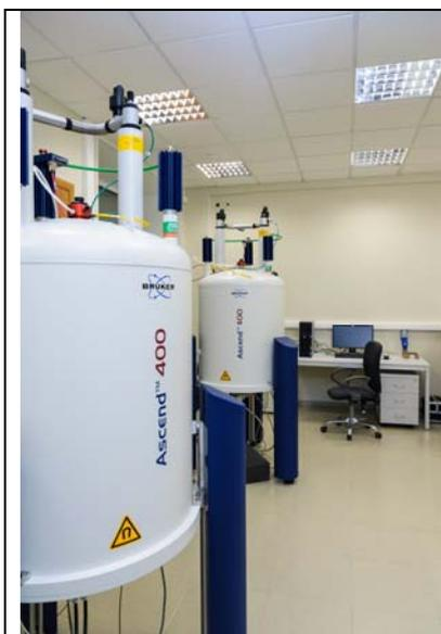
Bruker 300 MHz DPX and two Bruker 400 MHz Avance NMR spectrometers are dedicated to service routine measurements of 1D and 2D NMR spectra of liquids and solutions.
