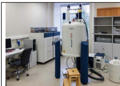
Bruker 500 MHz Avance NMR spectrometer is suited for measurements of 1D, 2D and 3D NMR spectra of liquids and solutions.
